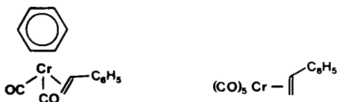
FIGURE 2 Proposed intermediates in styrene polymerization (Ref. 70c).
